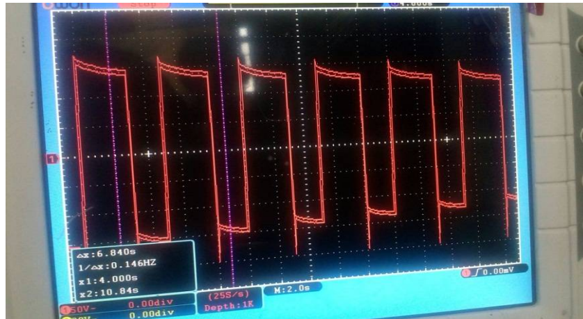
Fig.8.Output voltage of Inverter stage
